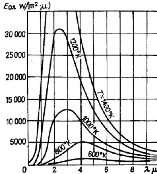
**Fig. 1.1:** Relationship of the monochromatic emission flux density of a perfect black body with wavelength and temperature.
