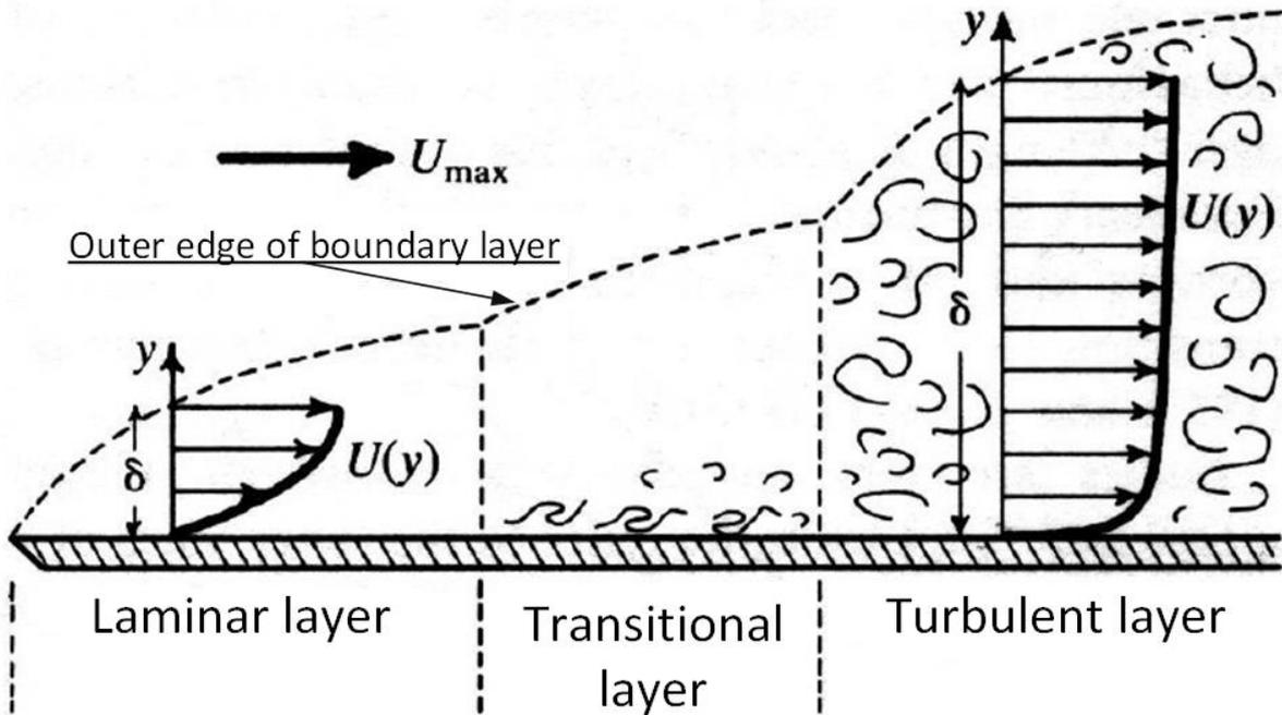
Fig. 1.3 Velocity distribution in the boundary layer
