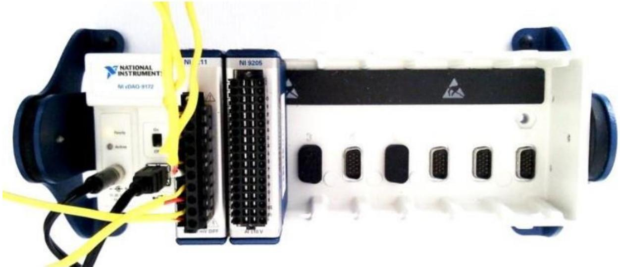
Fig. 4.2 Data Acquisition Module from National Instruments
