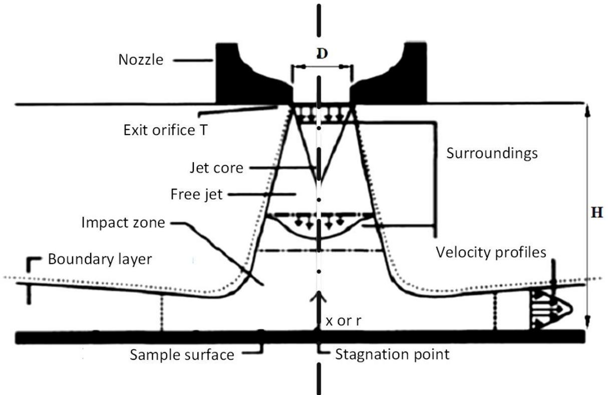
Fig. 2.1 Perpendicular Air Jet Impingement on the Surface
